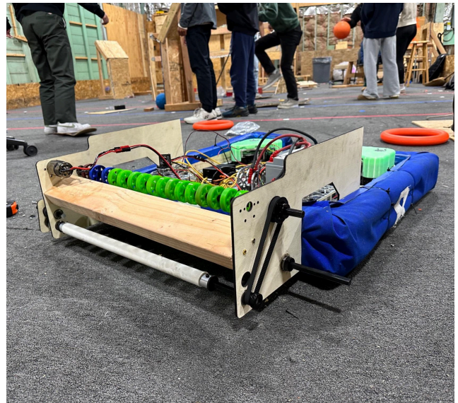
Intake Tested materials, roller placement, and several methods of passive vectoring (V-walls, dead-axle rollers).
