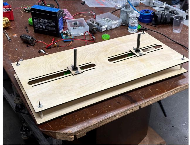
Double Flywheel Shooter Tested compression, wheel types, and velocity.
